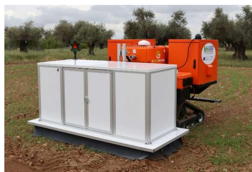
Fig. 1. Autonomous mobile system equipped with lasers for weed control.
